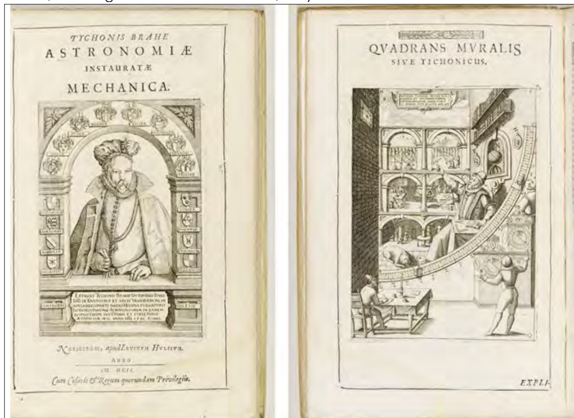
Fig.4/44 Tycho Brahe, Astronomiæ instauratæ mechanica , 2 nd edition 1602. Right - Brahe's mural quadrant, for measuring celestial bodies, seen as they pass across the small rectangular window, high on the left wall.
